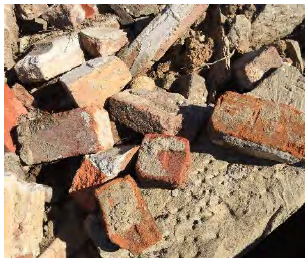
Figure 17 Hand cut stone, sandstock and dry pressed bricks with cement and lime mortar
