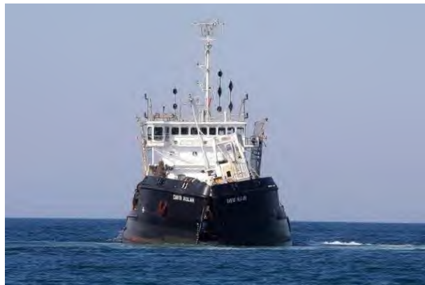
Split hopper TSHD, the David Allan, placing material at Stockton Beach in August 2018 (RHDHV, 2020; photo: Peter Cousins).
