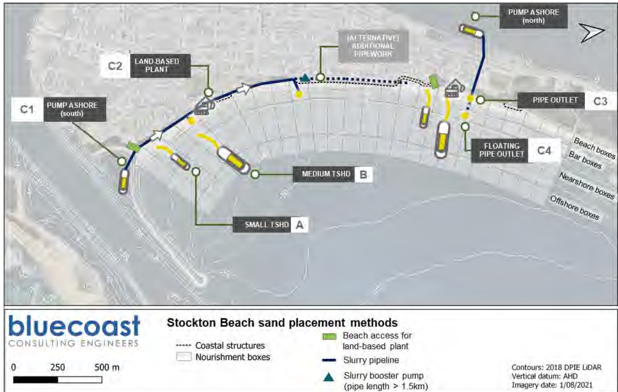
Figure 13: Conceptual diagram of feasible placement methods for beach nourishment at Stockton Beach.
