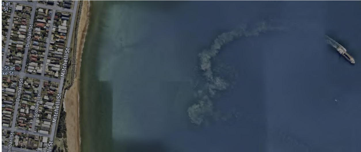
Figure 22: Aerial photograph capturing placement of nourishment material by David Allan on 23 April 2020 at Stockton Beach (source: Nearmaps).
