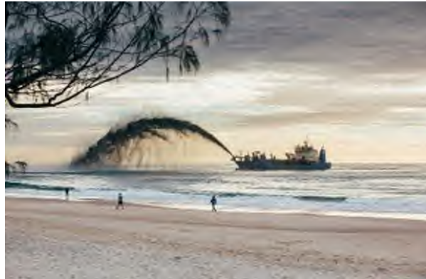
A medium sized TSHD rainbowing on the Gold Coast (source: City of Gold Coast).
