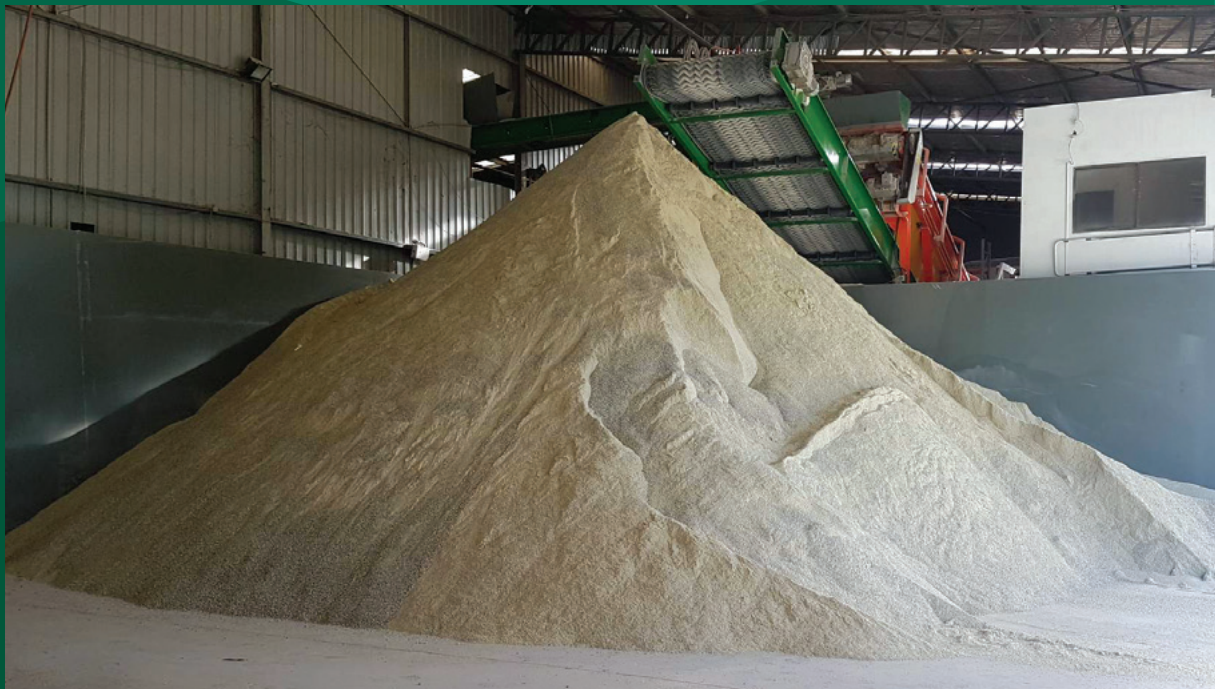
Glass collected from homes and businesses in Sydney’s northern beaches and the Central Coast is turned into sand - ready for re-use in road construction throughout NSW. However, more needs to be done to create markets for it in NSW.
