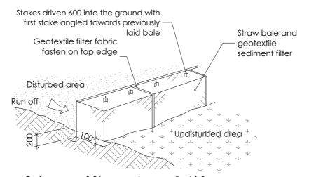
Drainage area 0.5 ha. max. slope gradient 1:2 max. slope length 50m.
