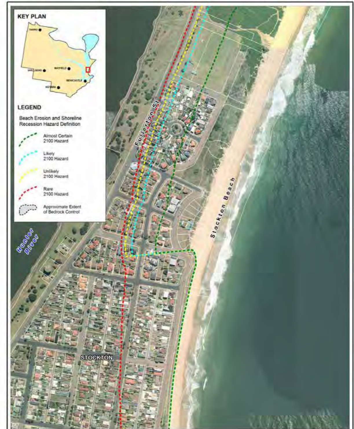
Title: Erosion and Recession Hazard Definition 2100 Planning Horizon - Stockton North Figure: C-3 Rev: A BMT WBM endeavours to ensure that the information provided in this map is correct at the time of publication. BMT WBM does not warrant, guarantee or make representations regarding the currency and accuracy of information contained in this map. 0 100 200m Approx. Scale BMT WBM www.bmtwbm.com.au Filepath : K:\N2051_NewcastleCoastalHazards&Management\MI\Workspaces\DRG_303_111025_Drawing_C-3.WOR
