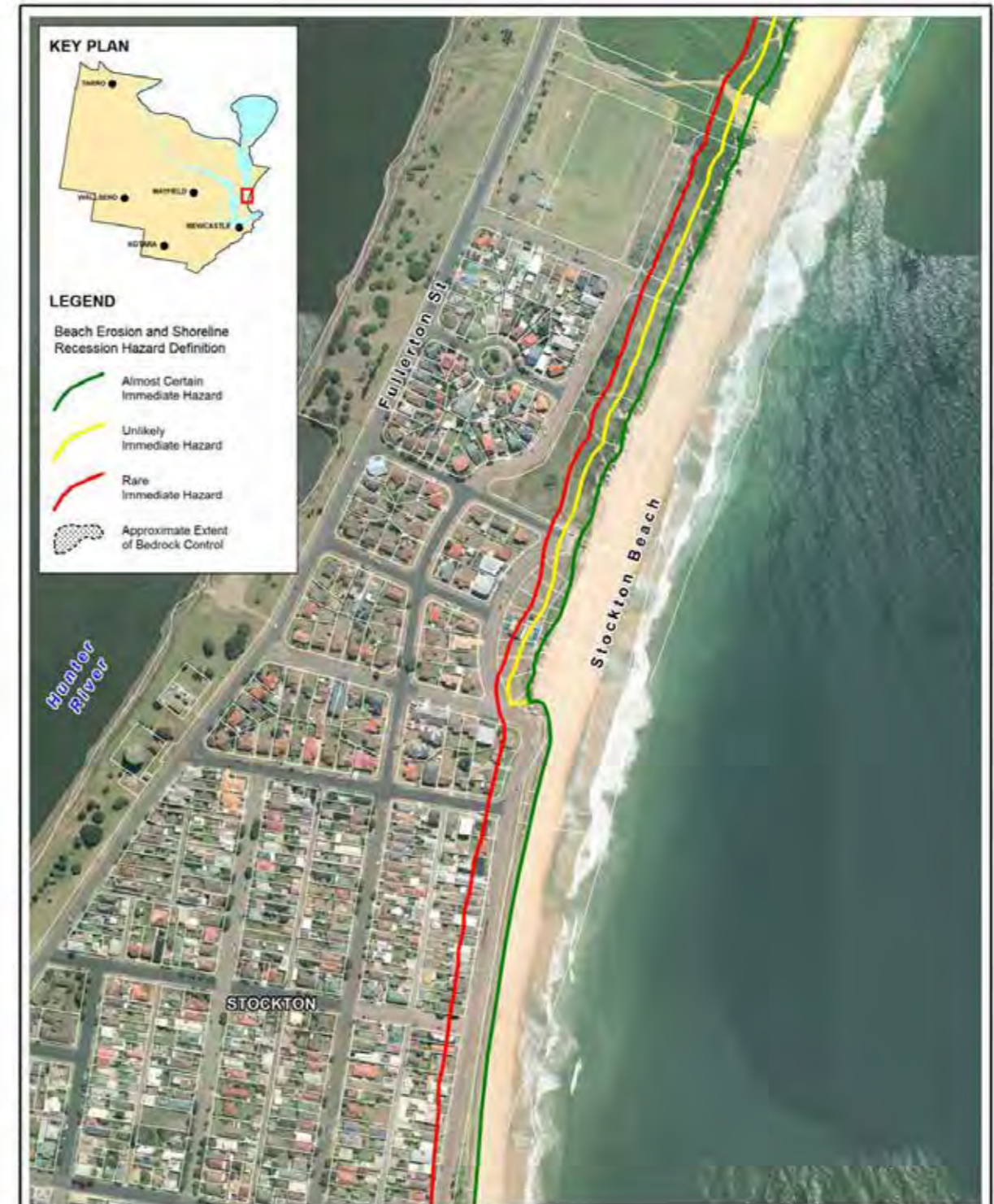
Title: Erosion and Recession Hazard Definition Immediate Planning Horizon - Stockton North Figure: A-3 Rev: A BMT WBM endeavours to ensure that the information provided in this map is correct at the time of publication. BMT WBM does not warrant, guarantee or make representations regarding the currency and accuracy of information contained in this map. Approx. Scale www.bmtwbm.com.au Filepath : K:\N2051_NewcastleCoastalHazards&Management\MI\Workspaces\DRG_103_111025_Drawing_A-3.WOR
