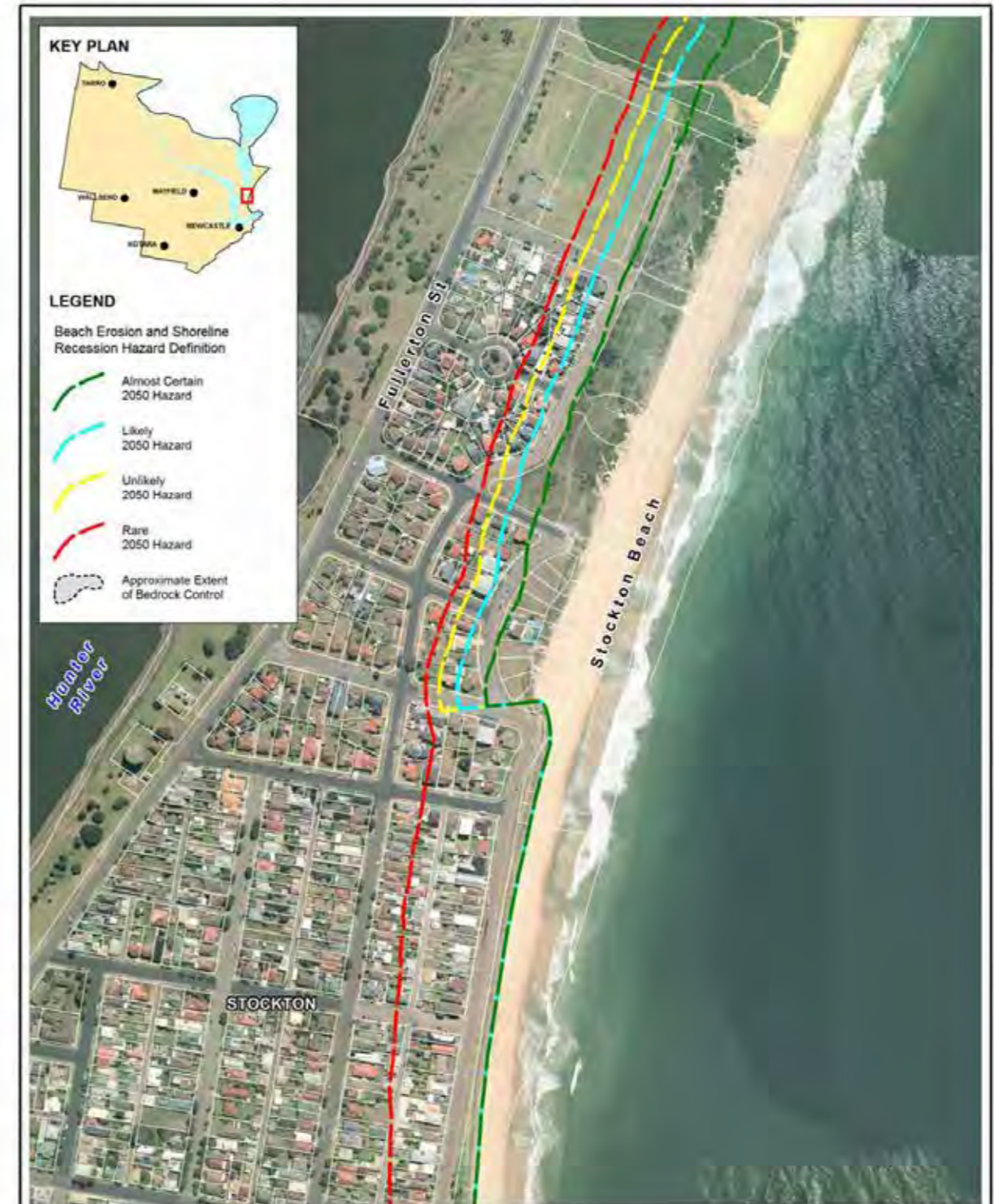
Title: Erosion and Recession Hazard Definition 2050 Planning Horizon - Stockton North Figure: B-3 Rev: A BMT WBM endeavours to ensure that the information provided in this map is correct at the time of publication. BMT WBM does not warrant, guarantee or make representations regarding the currency and accuracy of information contained in this map. Filepath : K:\N2051_NewcastleCoastalHazards&Management\MI\Workspaces\DRG_203_111025_Drawing_B-3.WOR
