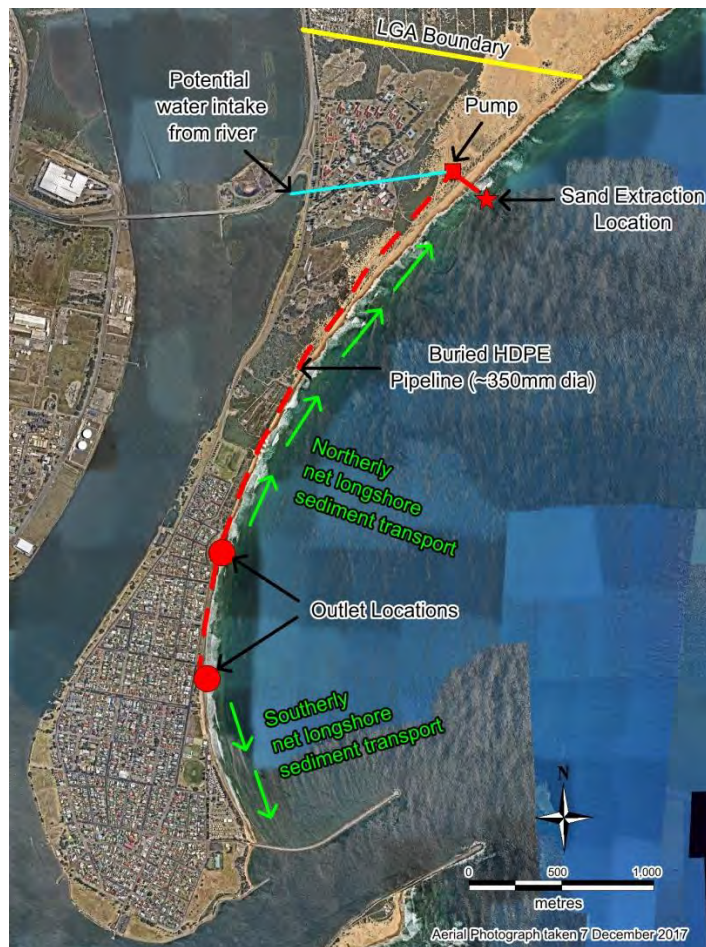
Figure 6: Sand backpassing schematic for Sand Shifter
