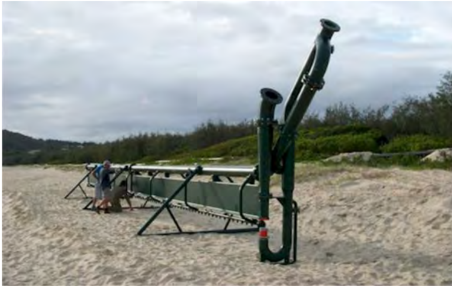
Figure 5: Example submerged sand extraction unit
