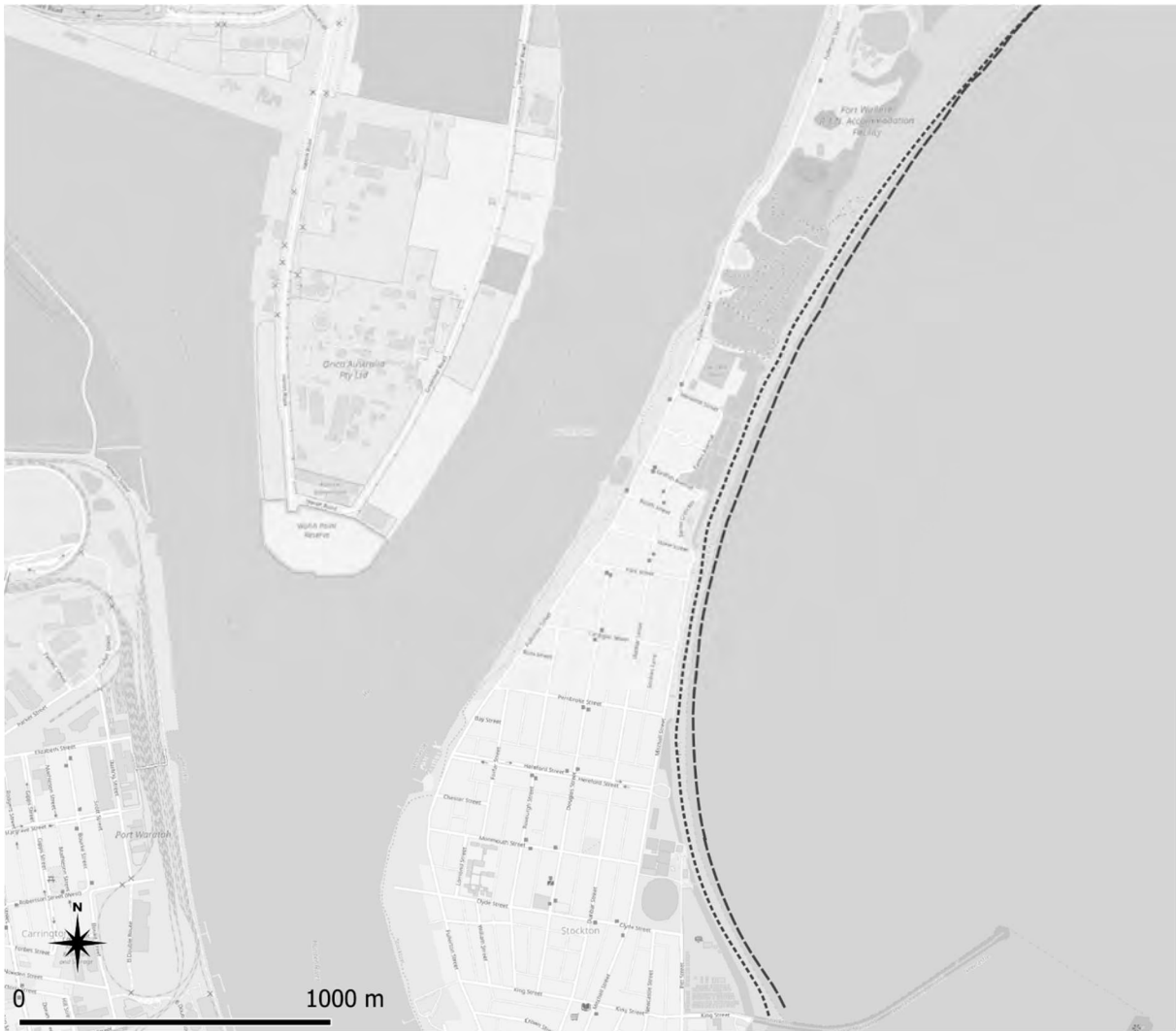
Figure 12: Mean sea level (0m AHD) shorelines from 2018 (inner) and 1994 (outer) showing realignment of the southern embayment.
