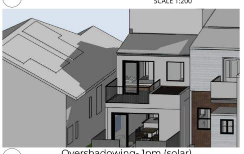
Overshadowing- 1pm (solar) SCALE 1:200
