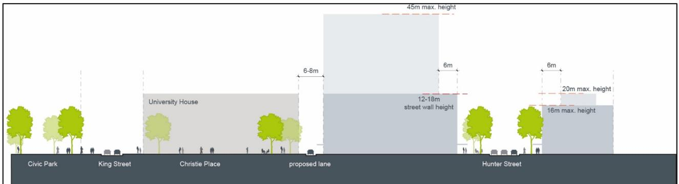
**Figure 6.01-36: Section through buildings fronting King Street and Birdwood Park showing 20m solar access plane setback**
