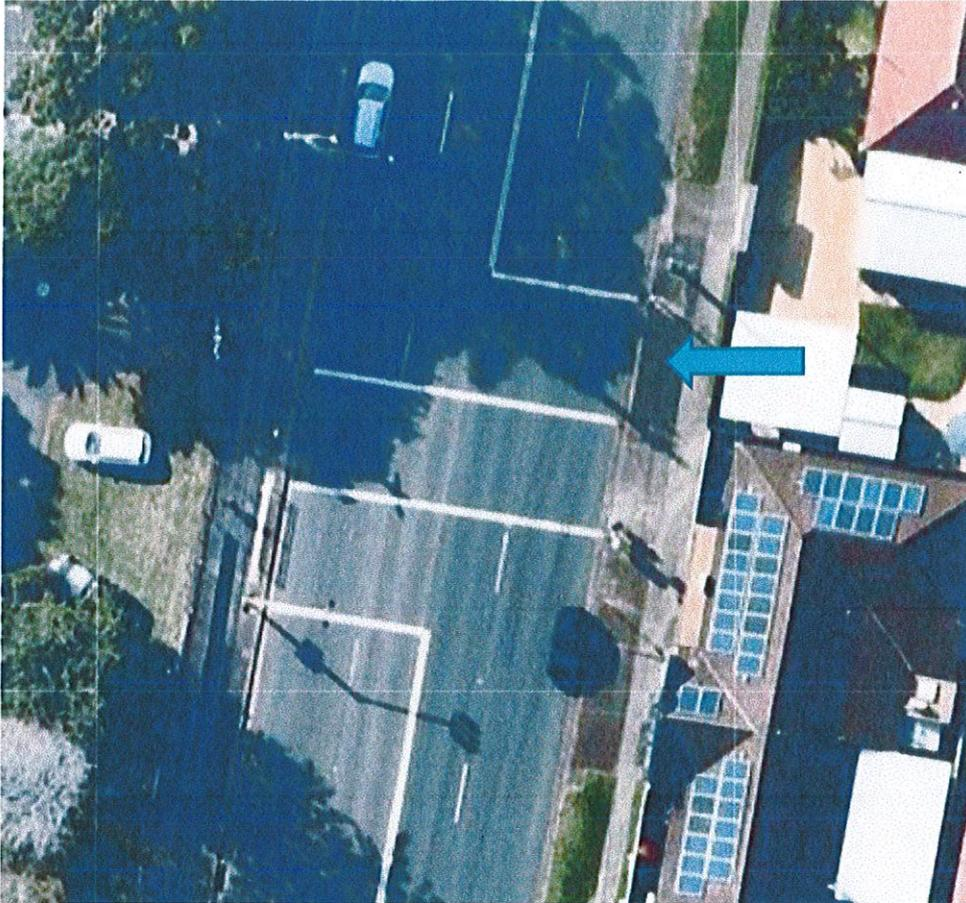
Figure 2 Aerial of pedestrian crossing showing uncontrolled area often treated by pedestrians as part of the crossing
