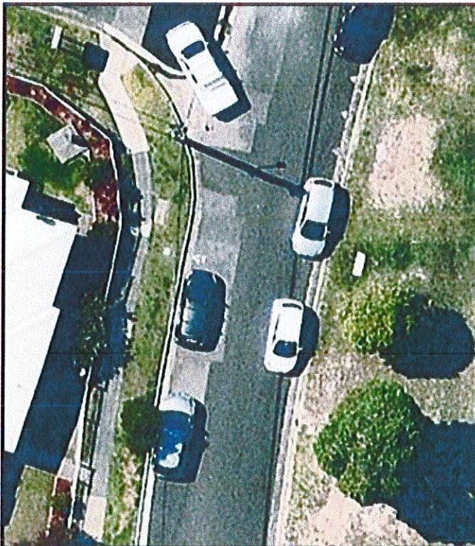
Figure 5 Existing uncontrolled parking creates road narrowing for 2-way traffic movements
