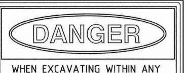
SITE, FOOTPATH AND ROADWAY, ALL SERVICES SHALL BE LOCATED PRIOR TO COMMENCEMENT OF THE EXCAVATION WORKS.
