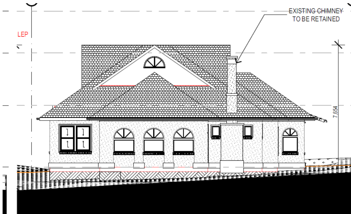
Figure 8: South elevation of existing dwelling showing current height, with the maximum height of 8.12m
