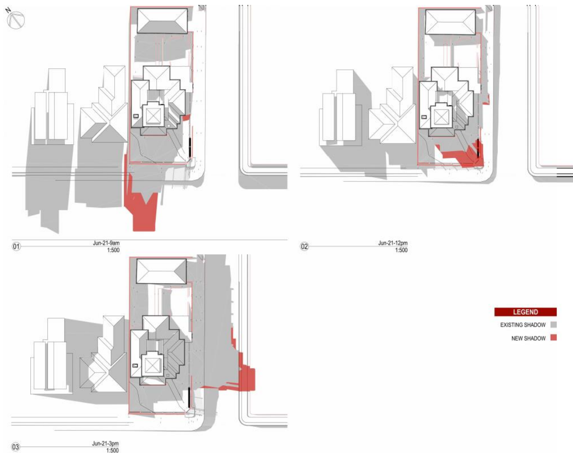
Figure 4: Shadow diagrams of the proposed development, with the impacts of the new additions shown in red (Source: EJE Architecture)
