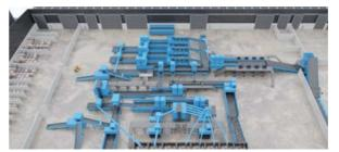
Layout of a Material Recovery Facility: A network of conveyors move the mixed recyclables through a series of equipment that sort the mixed recyclables into individual
