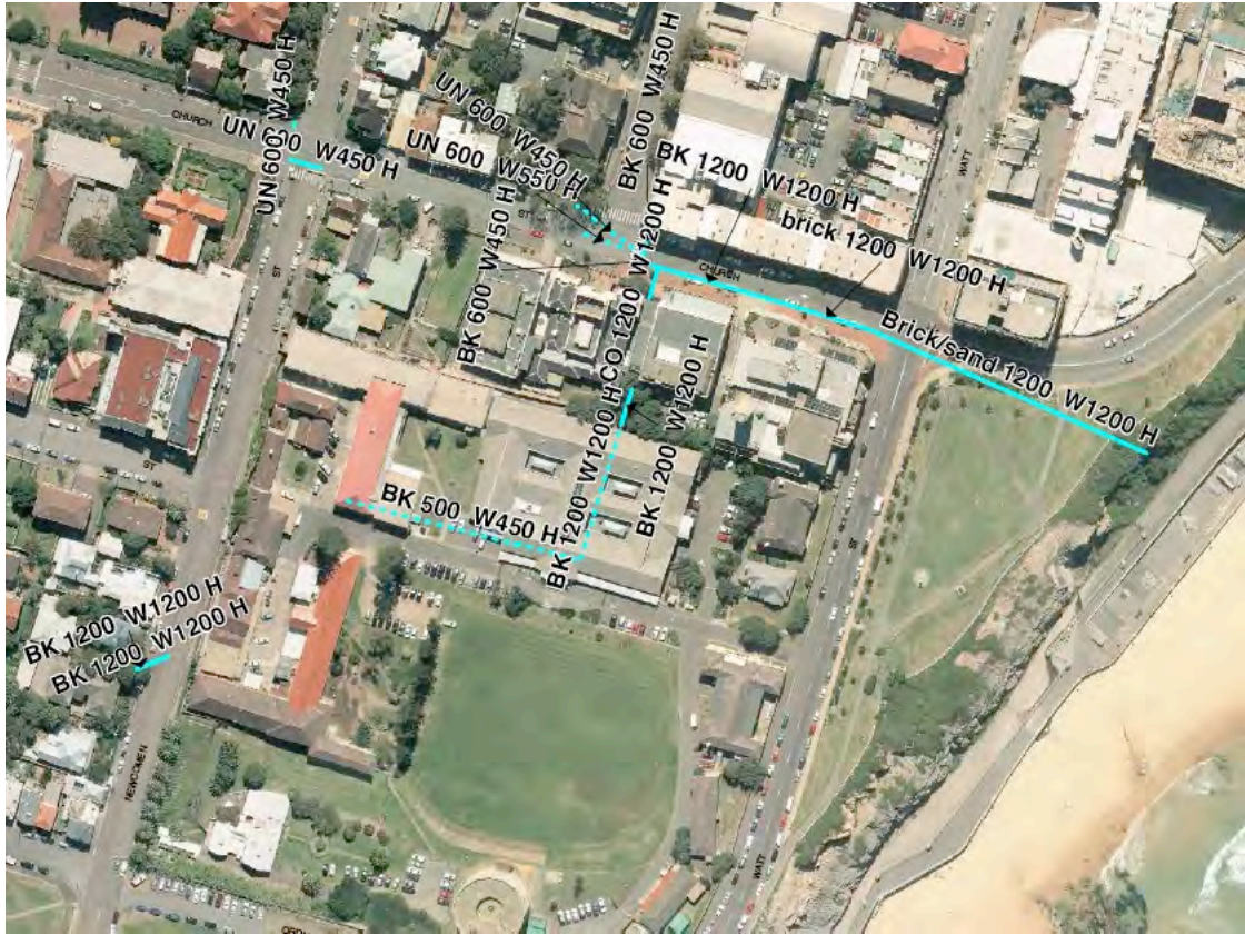
Newcastle City Council, 2012, Culverts 2 Aerial Photograph. Detail.
