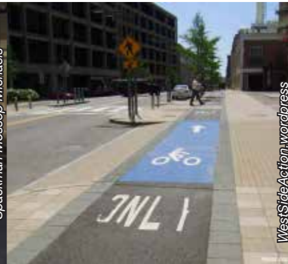
Raised pedestrian crossing over vehicular driveway access
