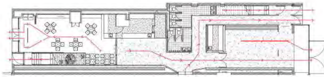
① 0 DOM - Ground Floor - Fire Exits 1:100
