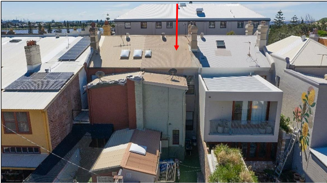
Figure 8 Existing rear setback conditions in the context of 37 Stevenson Place (indicated by red arrow). The rear setback of the proposed development will be approximately the average of no.33 (far right) and no.35. There are examples of further reduced setbacks in the lane including no. 41 (far left).
